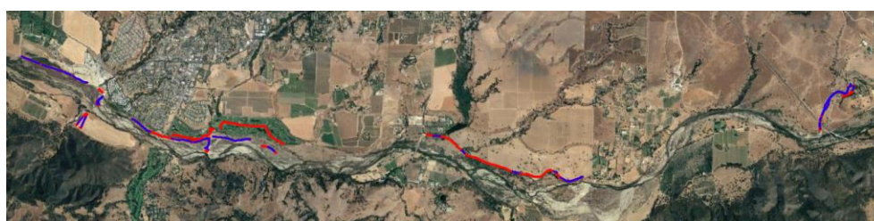
Figure 2 TTEM survey lines. The blue lines represents data used for inversion. The red lines represents data removed due to noise from man-made installations.
